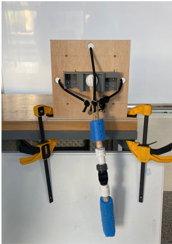
Fig. 1 ReducTrain assembly. Arm is in the healthy (i.e., non-dislocated) position for the traction-countertraction model. ReducTrain is attached to the table with two clamps
