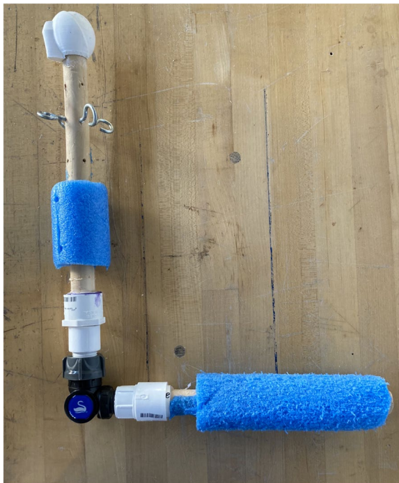
Fig. 4 ReducTrain arm assembly that is equipped with the 3D-printed humeral head, four screw eyes for tension band securing, swivel hose pipe adaptor, and cut pool noodles
